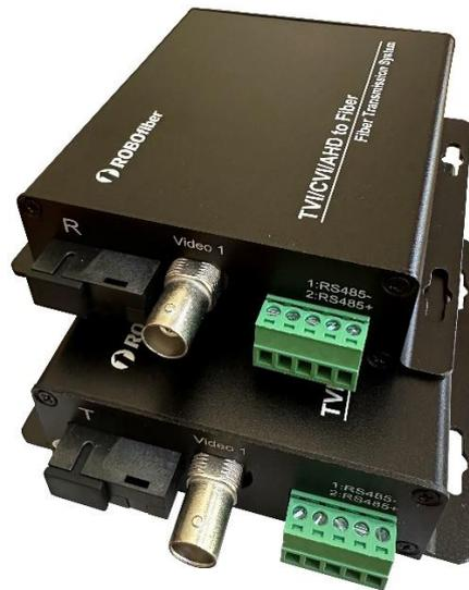
The RB-VIDEO-1D1 set is a one Channel Composite Video with one duplex data port that supports RS485, RS232 and RS422 protocols and extends video signal and data over one single strand of either multimode (62.5/125 or 50/125um) or singlemode fiber (9/125um).
